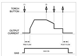
As shown above, it is possible to press and hold the TIG torch trigger a second time during downslope to end the downslope function and maintain the output current at the Crater current. When the TIG torch trigger is released the output will turn OFF and the postflow time will start. This operation, 2-step restart disabled, is the default setting from the factory.
